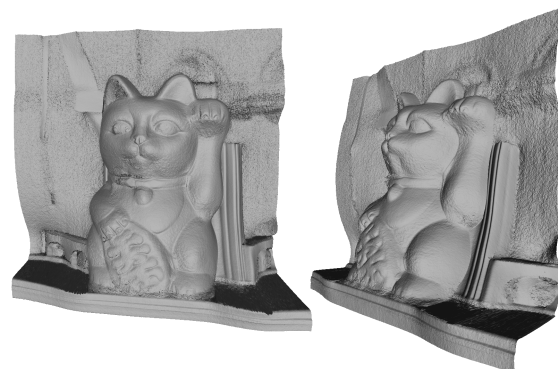
Figure 9: Reconstructed geometry for the cat subject, with normals derived from two photos instead of four.
