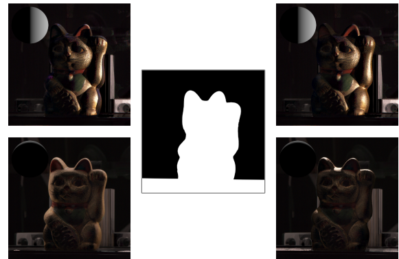
Figure 11: A user-supplied visibility mask (center) reduces unwanted shadows. Left column: Relit images under two point-light illumination conditions, no mask supplied. Right column: Mask supplied.
