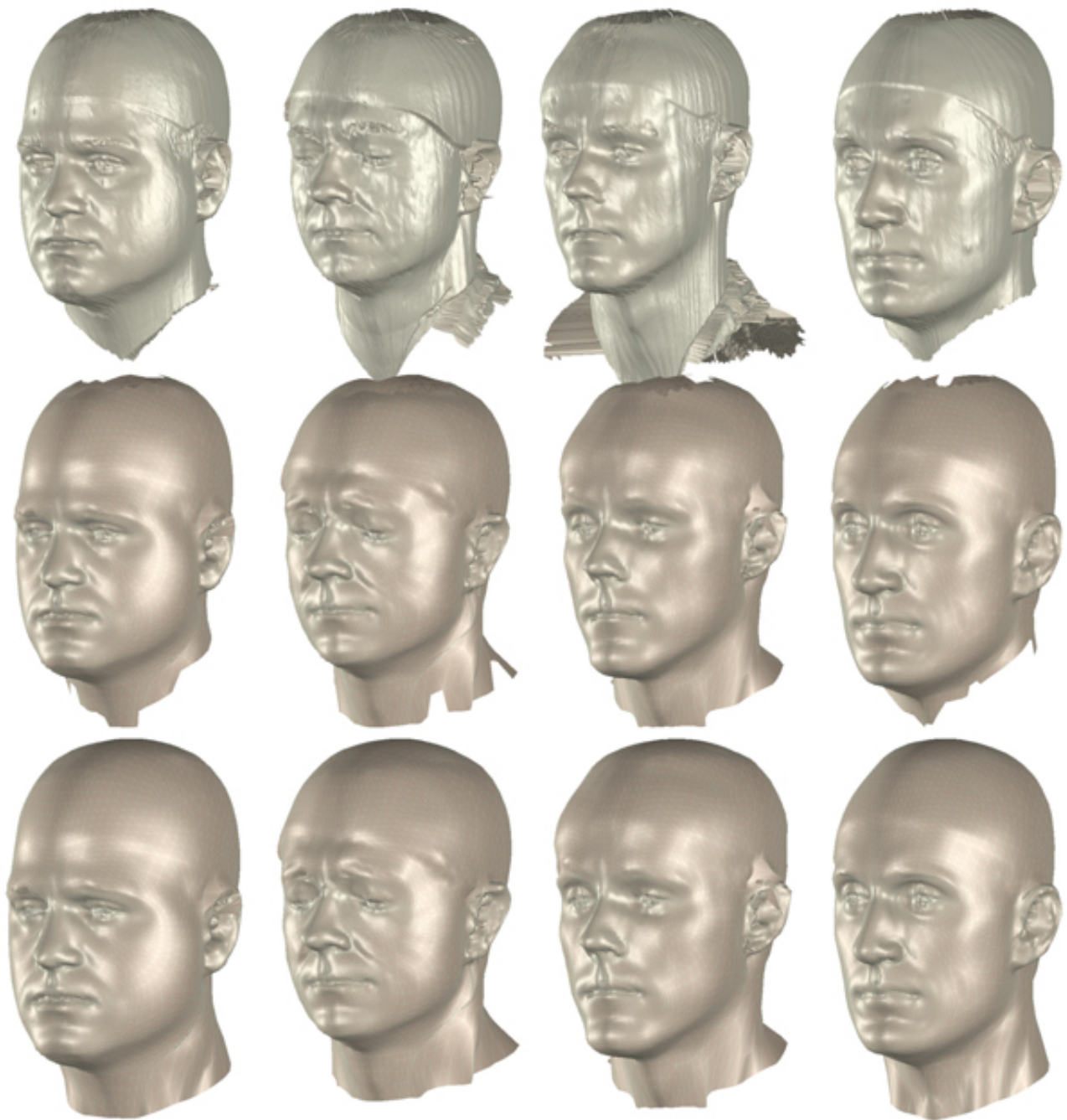
Figure 5: Results of the geometric registration algorithm. Top row: Original laser-scans. Middle row: Result after registration and topology transfer. Bottom row: Final result after hole-filling by offset interpolation.
