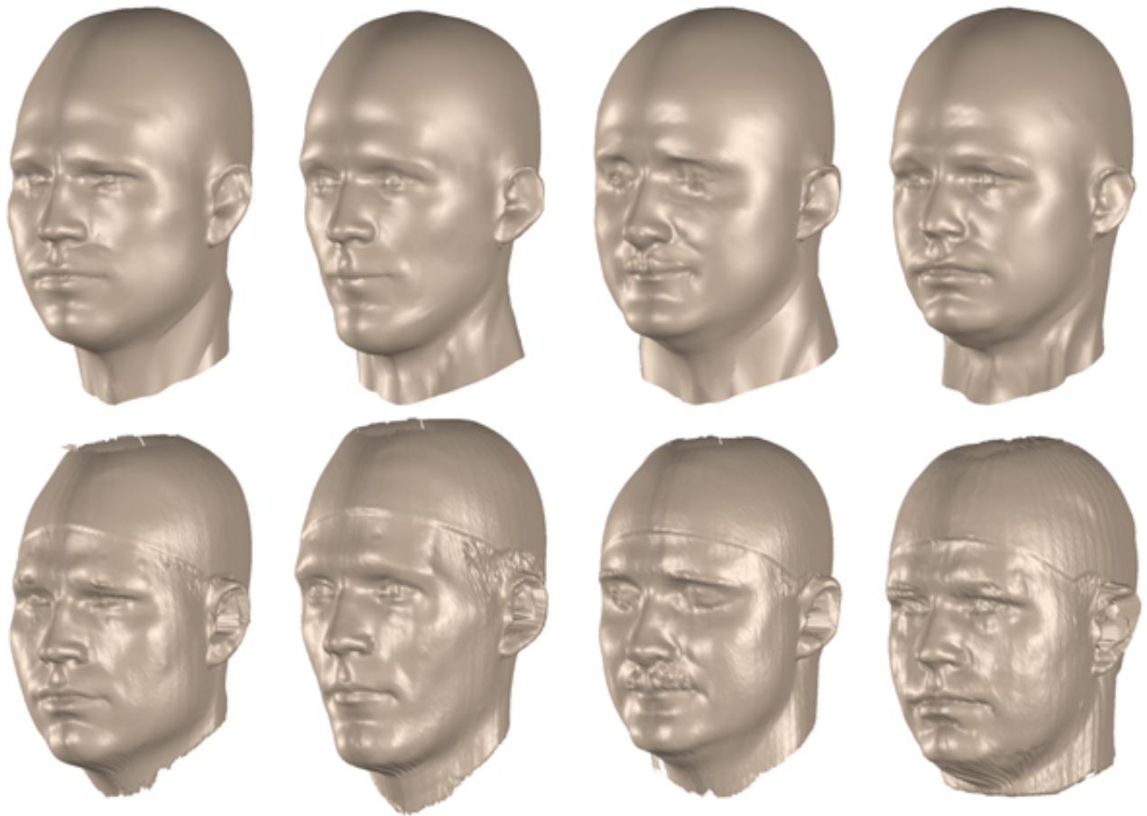
Figure 7: Results of the model-driven registration algorithm. Original laser-scans in the bottom row, fitted morphable model in the top row. Six region models and 15 principal components per region were used.
