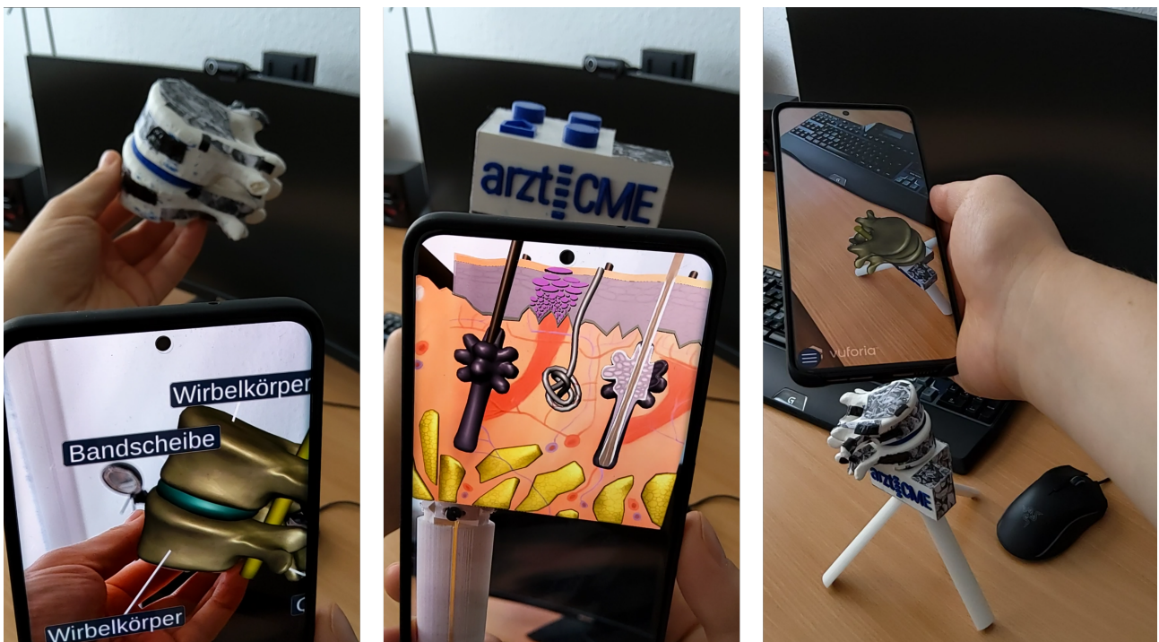
Figure 3: Prototype with the realistically shaped tangible interface (left), the generic tangible interface (middle), and the plug connection system interface (right).
