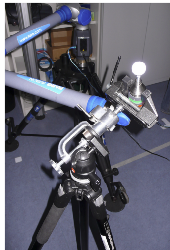
Figure 16: Fixed Faro tip with A.R.T. marker ball
