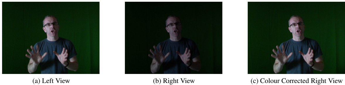
Figure 3: An example of the colour imbalance between the left and right views. (c) shows the right view after colour using the Pitić and Kokaram algorithm [PK07].
